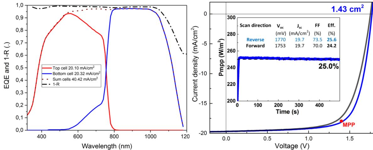
**Figure 4.** Tandem cell performances using a SHJ textured bottom cell. **Left:** External Quantum Efficiency measurement of top cell (red), bottom cell (blue), total current (dotted purple) and 1-Reflectance (dashed black). **Right:** current-voltage (IV) characteristics. The inset shows the MPP tracking over 10 min.
