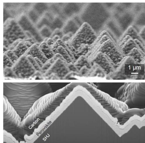
**Figure 5.** SEM image of the PK layer on top of the textured bottom cell. The lower image is a cross section obtained by focused ion beam. The carbon layer is here for protection purposes.
