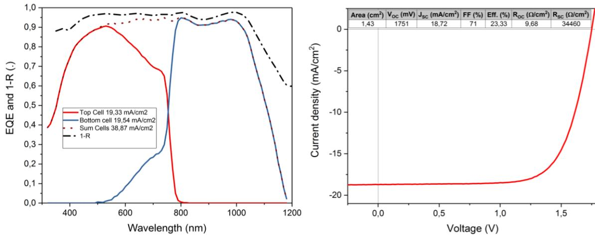
**Figure 3.** Tandem cell performances using a SHJ SST bottom cell. **Left:** External Quantum Efficiency measurement of top cell (red), bottom cell (blue), total current (dotted purple) and 1-Reflectance (dashed black). **Right:** current-voltage (IV) characteristics.
