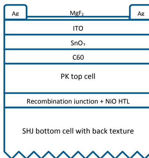
**Figure 1.** PK/SHJ tandem architecture using a SST bottom cell.
