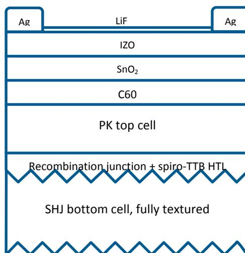
**Figure 2.** Tandem device with a textured bottom cell.
