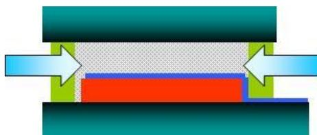
**Figure 2.** Important pathways for degradation of sealed perovskite device (adhesive).
