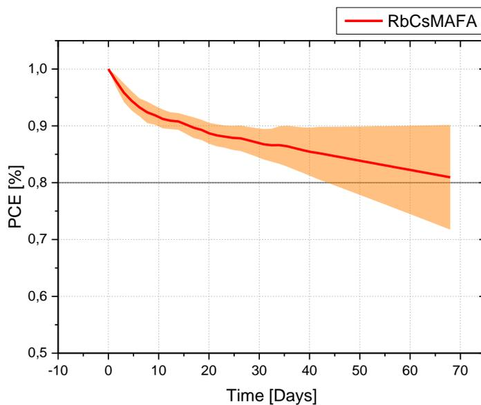
**Figure 16.** Degradation of perovskite solar cells made of RbCsMAFA of Fraunhofer IAP.
