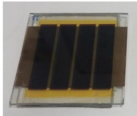
**Figure 13.** photograph of the encapsulated cells.
