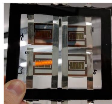
**Figure 14.** Photograph of the encapsulated cells.
