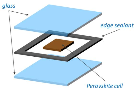
**Figure 15.** Sketch of the sealing procedure used by CSEM.
