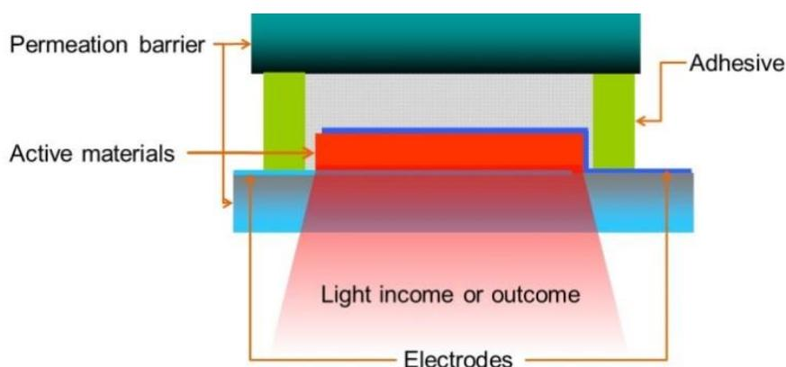
**Figure 1.** General set-up of an encapsulated device.
