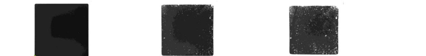
**Figure 9.** From left to right: Calcium-Mirror after 0 h, 72 h, 144 h (sample 160401117SK, 1 mm edge, storage at 60 °C und 90 % rel. humidity).
