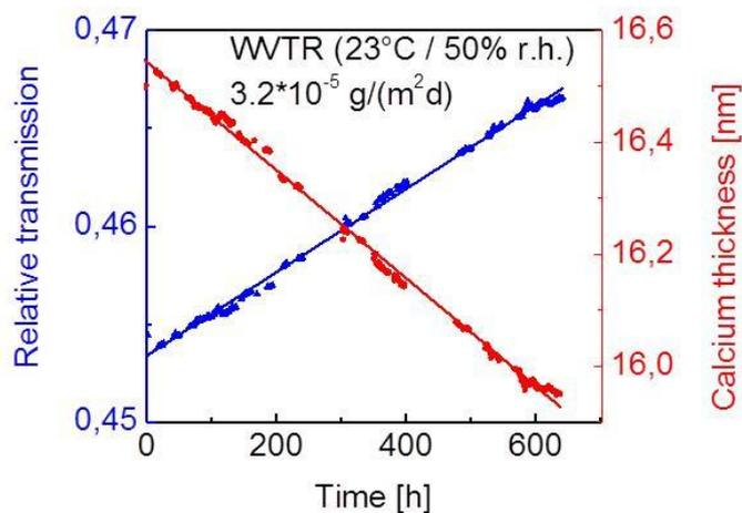
**Figure 4.** Determination of the water vapour transmission rate.
