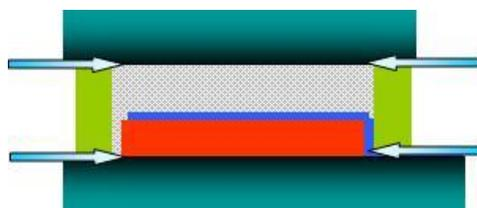
**Figure 5.** Important pathways for degradation of sealed perovskite device (Interface).
