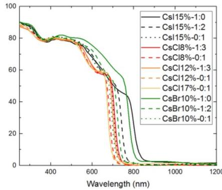
Figure 1: Absorbance spectra of different perovskite films on glass. Perovskites were obtained using different cesium precursors and evaporate rates (%) and varying the FABr:FAI (X:Y) concentrations.
