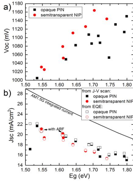
Figure 3: a)  $V_{oc}$  and b)  $J_{sc}$  of perovskite solar cells as function of their optical bandgap.
