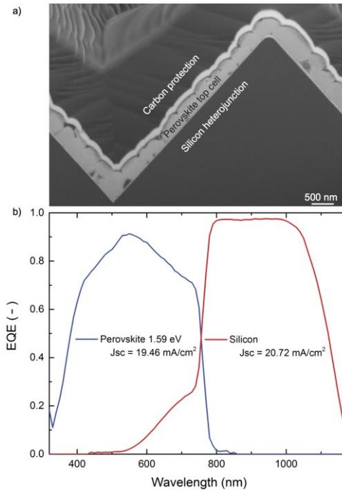
Figure 4: a) SEM image of the cross-section of a textured tandem prepared using a focused ion beam, b) external quantum efficiency (EQE) of a textured perovskite/silicon monolithic tandem. The perovskite bandgap is 1.59 eV.
