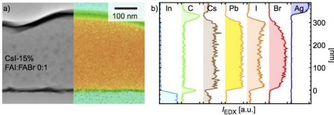
Figure 2: a) Scanning TEM micrograph and corresponding EDX map of a perovskite cell produced by co-evaporating CsI and  $\text{PbI}_2$  precursors, b) background-subtracted intensity profiles of the different elements present in the cell.
