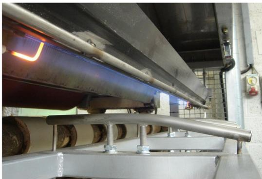
Figure 1: Photograph showing a production flame treatment system
