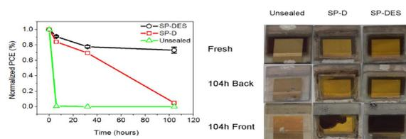
PCE behavior and images during the damp-heat test with and without sealing process
