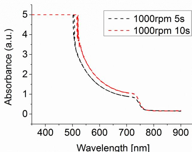
**Figure 5.** Comparison between absorbance spectra by varying the spin coating program.
