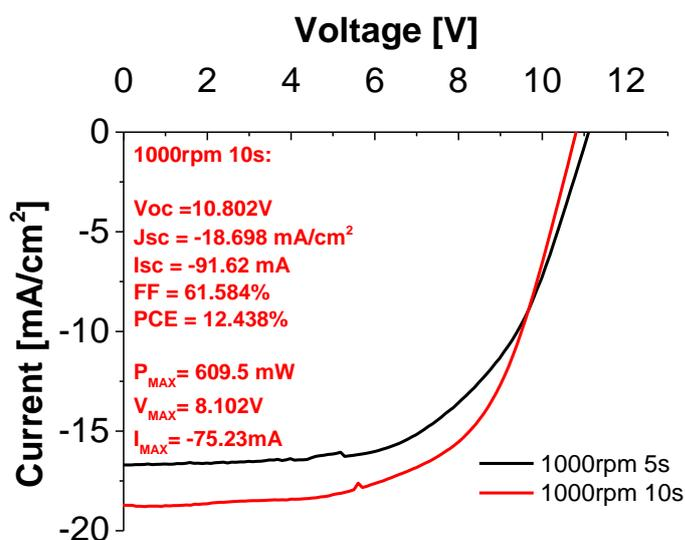
**Figure 6.** I-V curves of the modules by varying the spin coating program: 1000 rpm 5s (black curve) and 1000rpm 10s (red curve).
