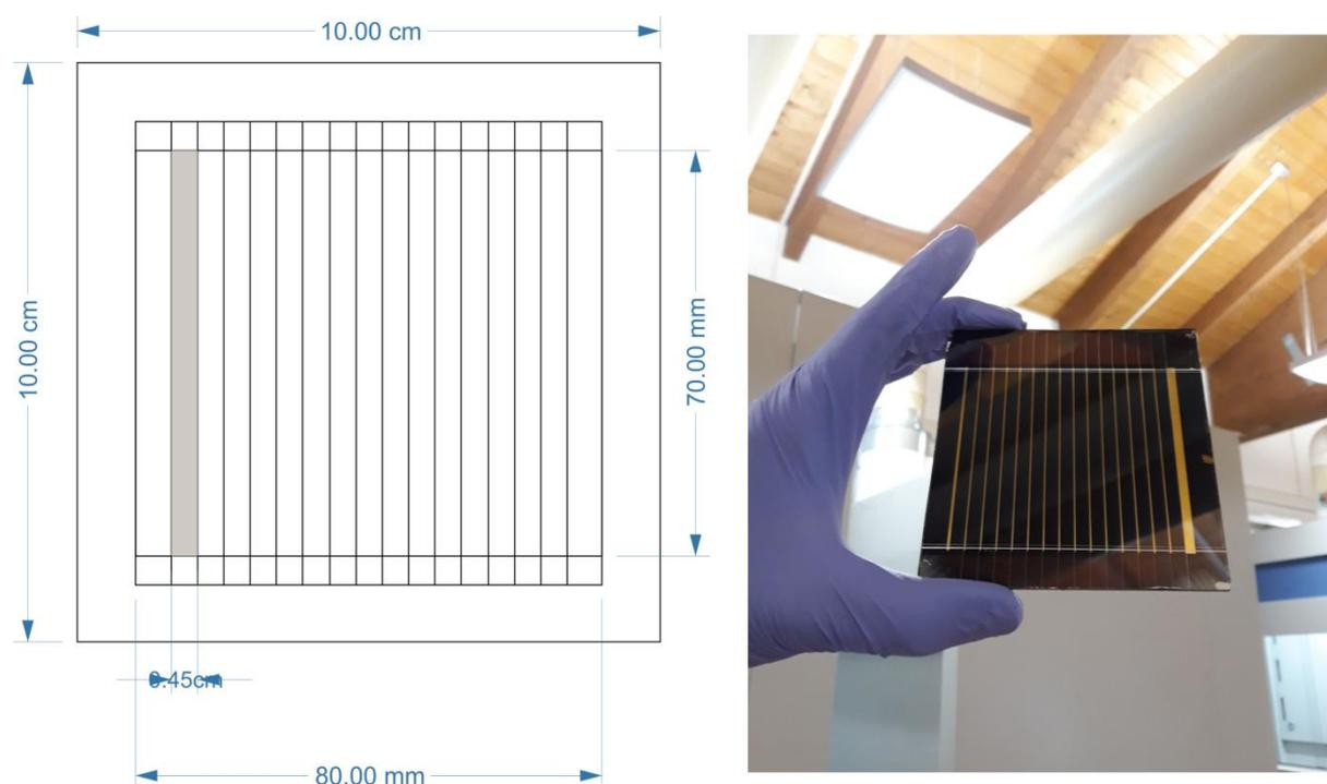
**Figure 7.** Optimized layout for planar PK modules with 4.5mm cell width and 15 cells.
