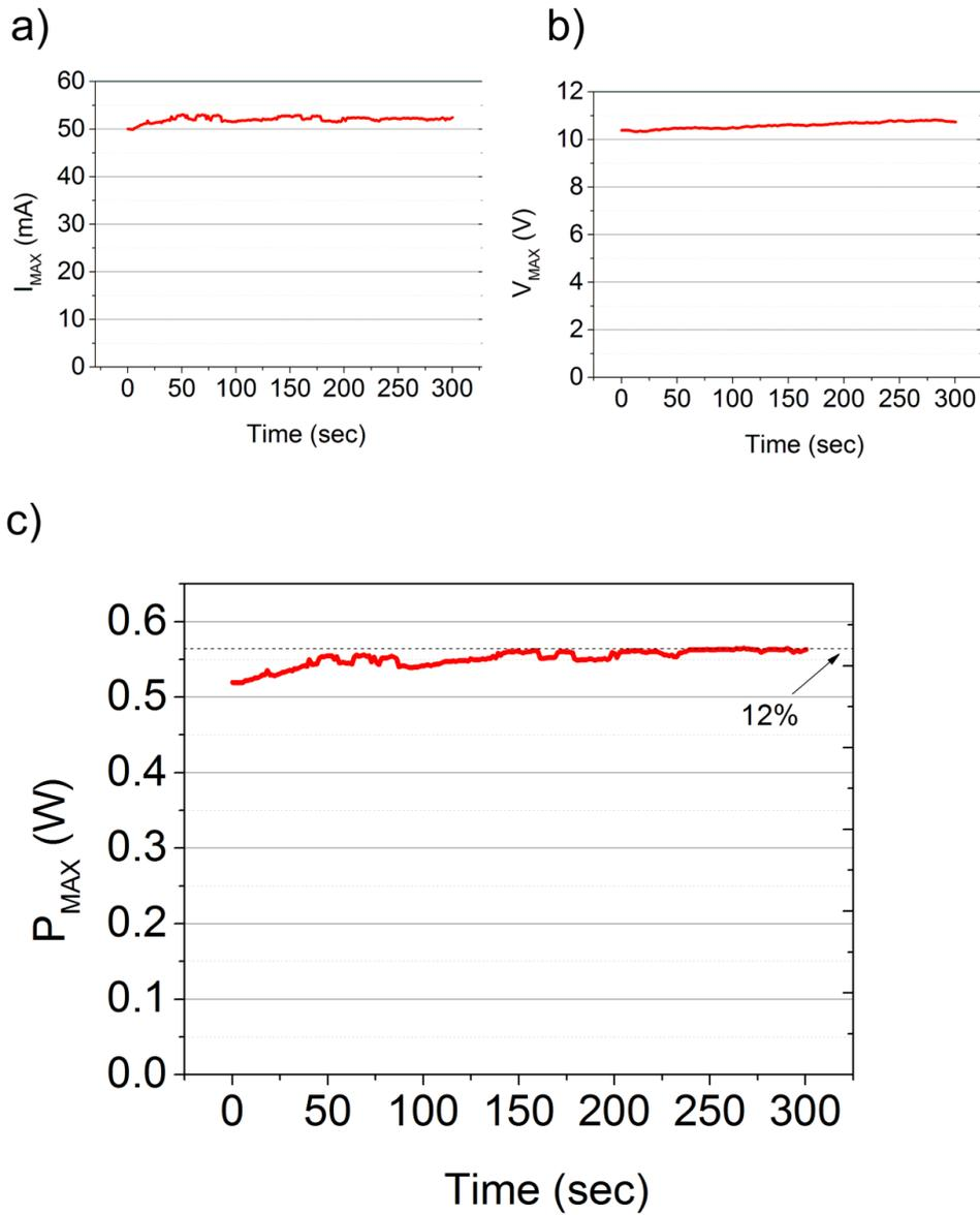
**Figure 9.** Results obtained for MPPT test long 300s: a)  $I_{MAX}$  profile, b)  $V_{MAX}$  profile, c)  $P_{MAX}$  profile.
