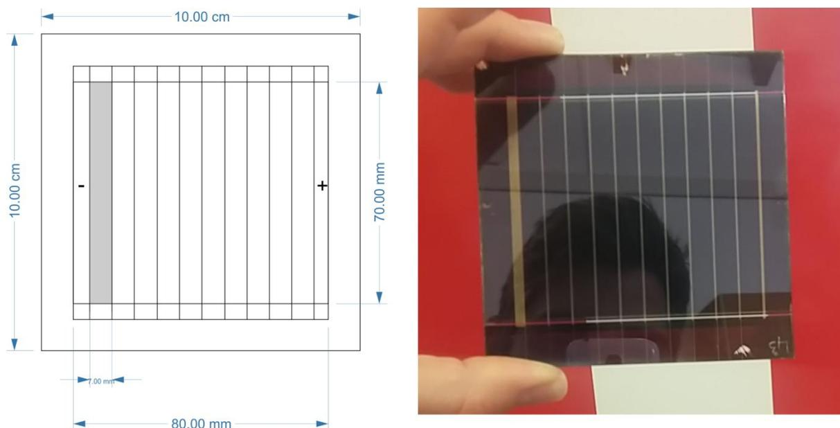
**Figure 2.** Layout of the PK module formed with 10 sub- cells. Each cell has a 7mm width and a 70mm length. The series interconnections are obtained by P1-P2-P3 laser ablation.
