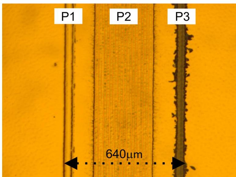
**Figure 3.** Image of the monolithic interconnection of the modules. The total dead area width was around 640μm.
