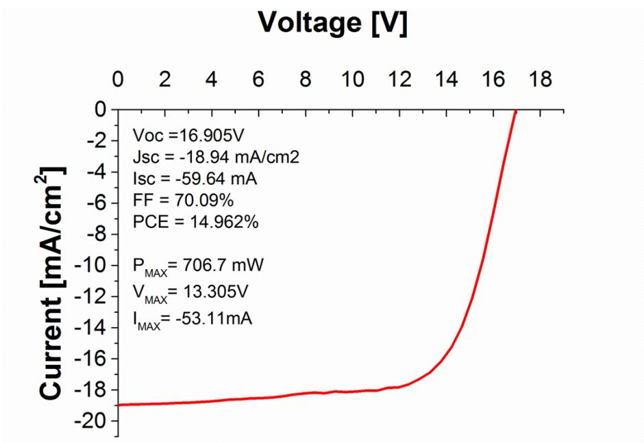
**Figure 8.** I-V characteristic of the optimized module.
