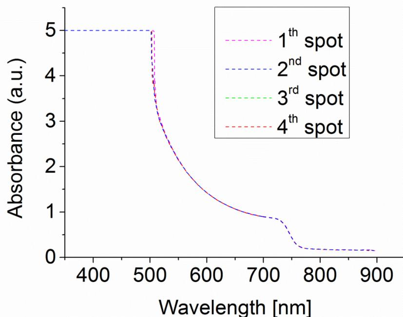
**Figure 1.** Absorbance spectra of the module in four different spots of the 10x10cm<sup>2</sup> sized device.
