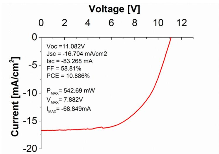
**Figure 4.** I-V curve for planar PK module with 7mm as cell width.
